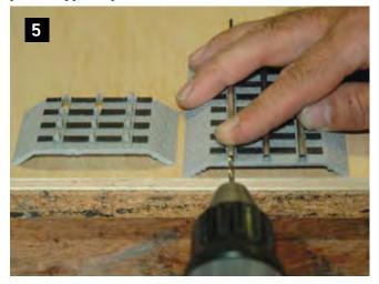
rail. These can be seen if you look at the small section to the left of the track being drilled in **photo 5**. Drill to a depth of at least one half the length of an O-gauge track pin. Be sure to keep the drill against the inside top of the rail and support the rail from above with your finger.
