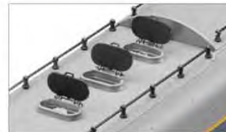
Prototypical tender features easy-to-access RailSounds controls under water hatches
