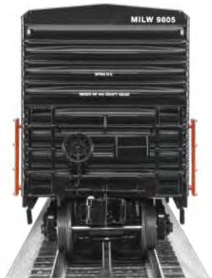
Realistic details including modern low brake equipment and short ladders
