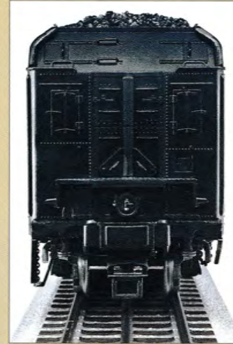
Tender includes separately applied coal and directional lighting
