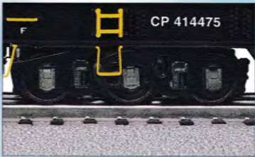
CP 414475 Die-cast metal 6-wheel sprung and equalized trucks
