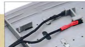
Wire attached to terminal
