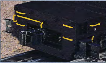
Remotely deployed outriggers and front and rear ElectroCouplers
