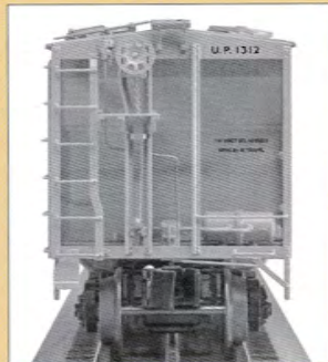
Die-cast metal end platforms
