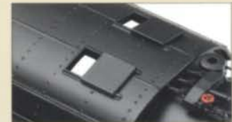
New opening roof hatches
