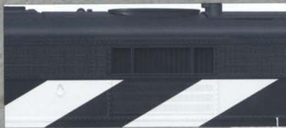
Auxiliary cooling vents for steam boilers
