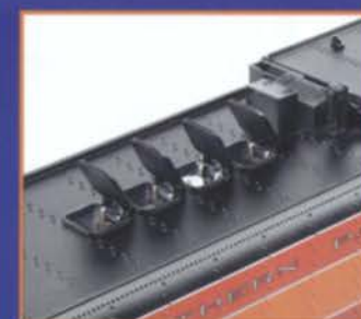
Opening tender water hatches reveal RailSounds controls
