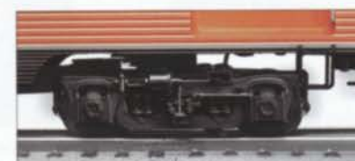
All-new die-cast metal sprung trucks
