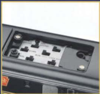
Removable roof panel reveals GG1 controls
