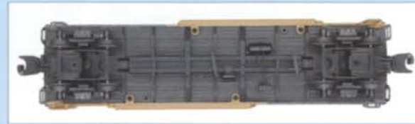
Separately applied metal underframe details
