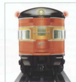
Illuminated marker lights, end light and drumhead
