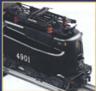
Distinctive vent details with opening roof hatches, end doors and cab doors
