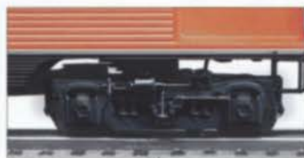
All-new die-cast metal sprung trucks
