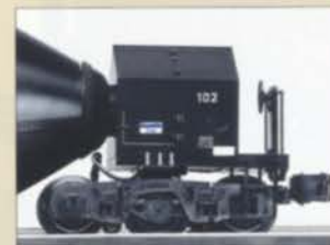
Fully equalized die-cast metal sprung trucks
