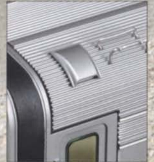
Detailed, fluted roofs include metal vents and grab handles
