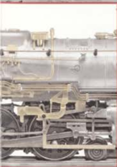
Many separately applied metal detail parts
