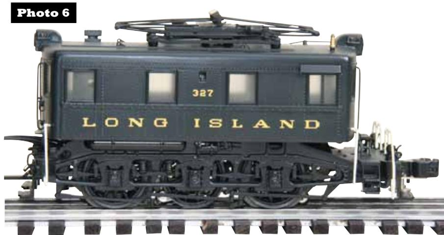
Box Cabs. Return with me to The Standard Railroad of the World, the mighty PRR, and look at its smallest electric loco, the B-1. This little switcher originally operated in semi-permanently mated pairs, later as single units. See photo 6. Its proportions just about match those of the toy versions. It has only one truck,
