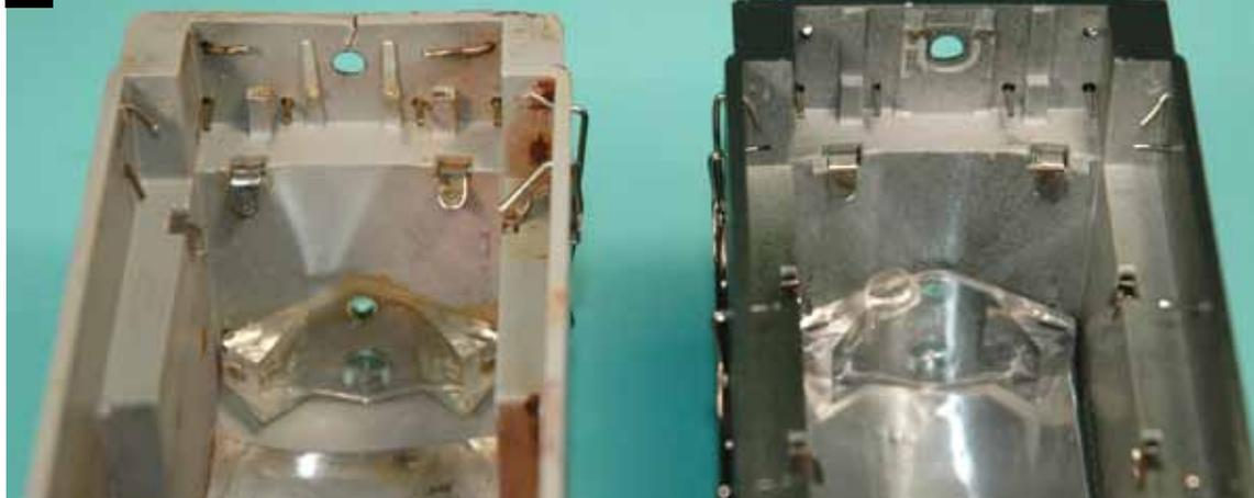
**Photo 8** illustrates the changes made to the male portion of the die to correct the problem. The postwar Lackawanna is on the left. As you can see, several changes were made. The area at the screw hole has been made thicker and the four vertical spacers have also been thickened and extended. I cannot verify exactly when these changes were made to the shell.
