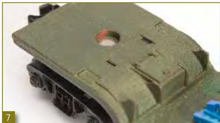
**Photo 7** details the circular area where the plastic AAR truck was riveted directly to the car body. Look closely, and you will notice an area of red that was not completely covered during the painting process.
