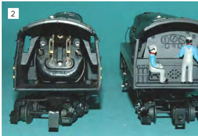
along with several visual improvements. **Photo 2** shows the cab of the original 746 on the left and the latest version on the right. Although the new one still features a Pullmor™ motor, it has been shielded with a detailed cab interior. It has a red firebox glow, and an engineer and fireman are on duty.
